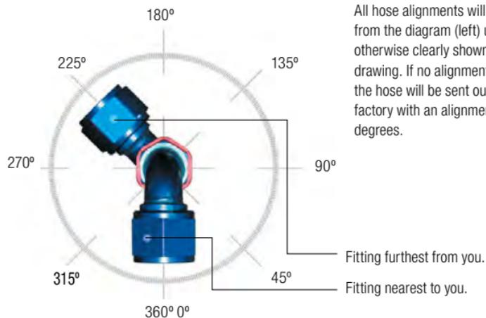
All hose alignments will be taken from the diagram (left) unless otherwise clearly shown on a drawing. If no alignment is stated the hose will be sent out of the factory with an alignment of 0 degrees.
